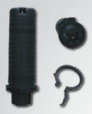
GPJM5-RS provide with six fiber cable in-out ports (4 round ports, 1 elliptical port), it can be used in aerial and underground application, it is made from quality engineering plastic, the cover and the base are filled with silicon rubber and sealed with hoop, then entry ports are sealed with heat-shrinkable tube, it can be opened after sealing and can be reused without changing sealing material.
